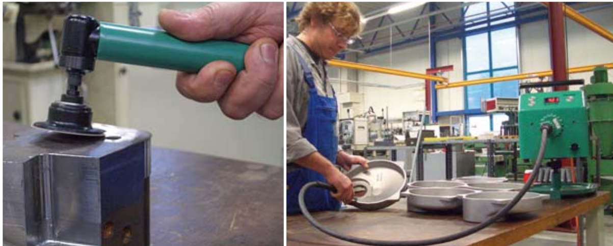
MBF 5 Z For light and heavy deburring-, cast cleaning- and wive brushing work.
